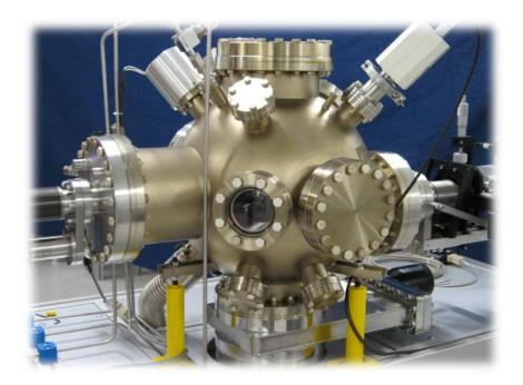
Synthesis of complex materials & crystalline structures is a constant growing request from the research. Pulsed Laser Deposition (PLD) is one answer. It is a versatile coating technique that allows the growth of various materials as nitrides, oxides, superlattices, polymers, composites...
